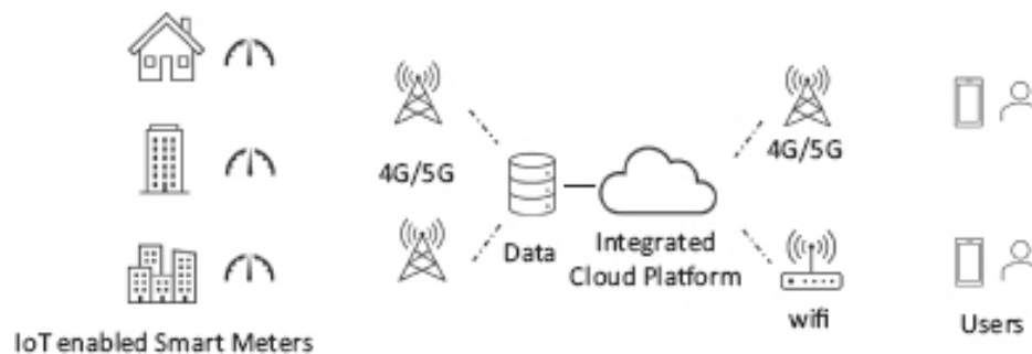
Figure A.16 Smart Metering solution
