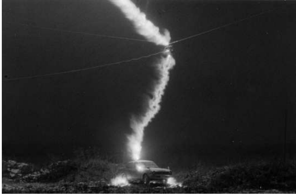
Triggered-lightning strike to a fully enclosed car with a live rabbit inside. The strike terminated on the radio antenna. The rabbit inside the car was not harmed. Note flashovers across the tires (which were not damaged) and ground surface arcs. Courtesy of S. Sumi.
